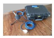
Once you have finished doing your recording and have pressed the reference tone marker, simply close the case with all wires coming out of the slot in the side and apply the padlock. Place the case in the room where the person is complaining of greatest disturbance, making sure the microphone is not touching any surfaces
