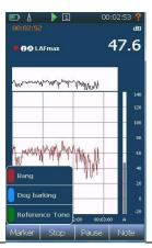
To add a reference audio recording to your file simply press the 'marker' button at the bottom of the screen and select the 'reference tone' marker. If this is not present then it can be activated by going into 'Set-up' and 'Marker' and selecting one of the 9 available markers to be used as a reference tone.
