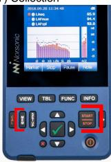
Open the case. If the meter is still running press the 'Stop' button either on the screen or keypad. If your meter is set to 'Automatic' saving, then the file will have been saved as the date it started.
