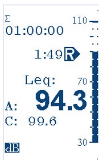
The sound level meter display shows both A- and C-/Z-weighted levels simultaneously
